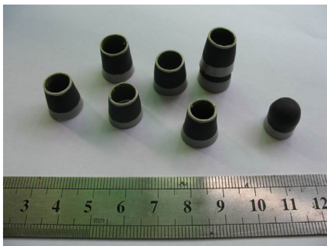
Fig. 3. The photo of the cone-shaped anode-supported SOFCs.
